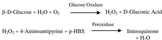
$\beta$ -D-Glucose is oxidized by glucose oxidase to produce D-gluconic acid and hydrogen peroxide. The hydrogen peroxide is then oxidatively coupled with 4-aminoantipyrine and phenol substitute, p-HBS, in the presence of peroxidase to yield a red quinoneimine dye. The amount of colored complex formed is proportional to glucose concentration and can be photometrically measured.
